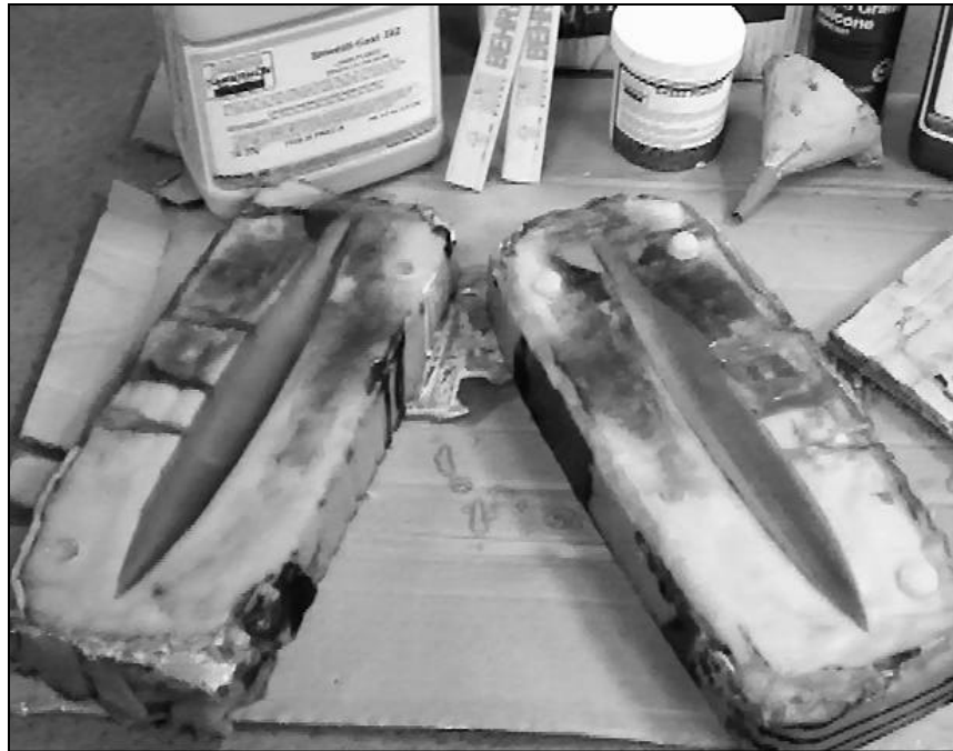
Figure 9. Finished Rubber MK-84 Model Mold
