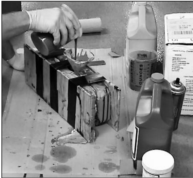
Figure 10. Pouring the Resin Mixture into the Model Mold
