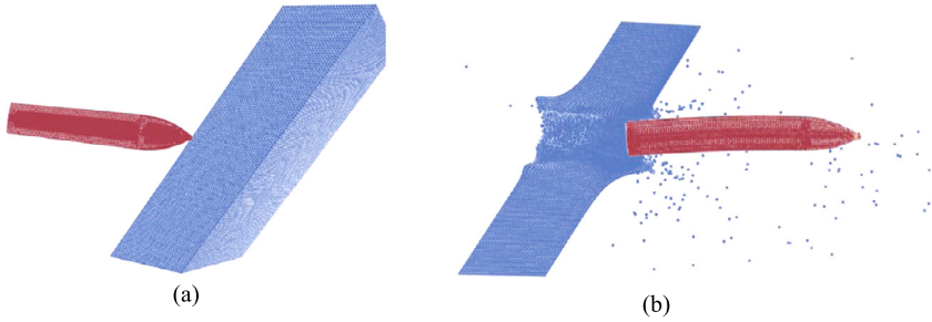
FIGURE 3.22 MPM models for simulating oblique penetration.
