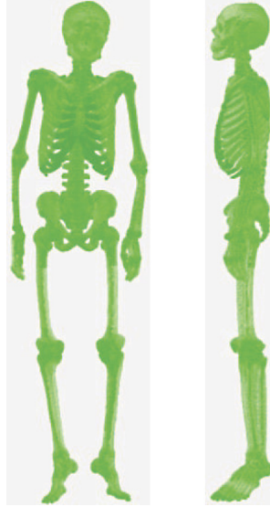
FIGURE 8.24 The MPM model of the human body generated by CT-scanned images: (left) front view; (right) side-view.
