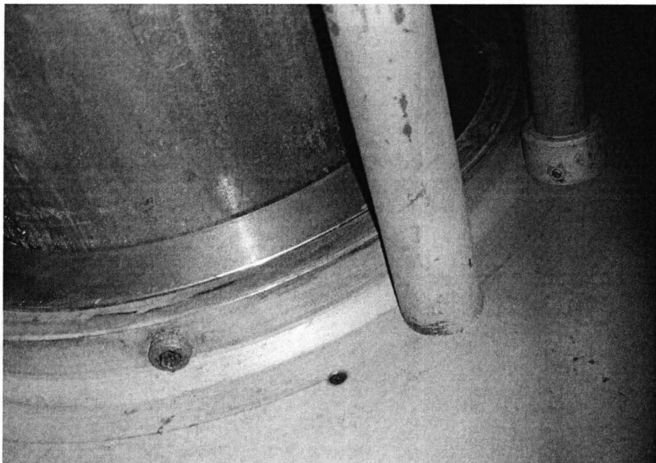
This photo shows the 8" steel pipe that the DOE later substituted for the original gun tube in this LB. The newly-manufactured steel filler bushing is visible between the pipe and the locking collar. The primer wire tube is shown on the far right and the 1.0" steel rod used to attach the tail section to the bulkhead plate is also visible in the foreground. (Author)
