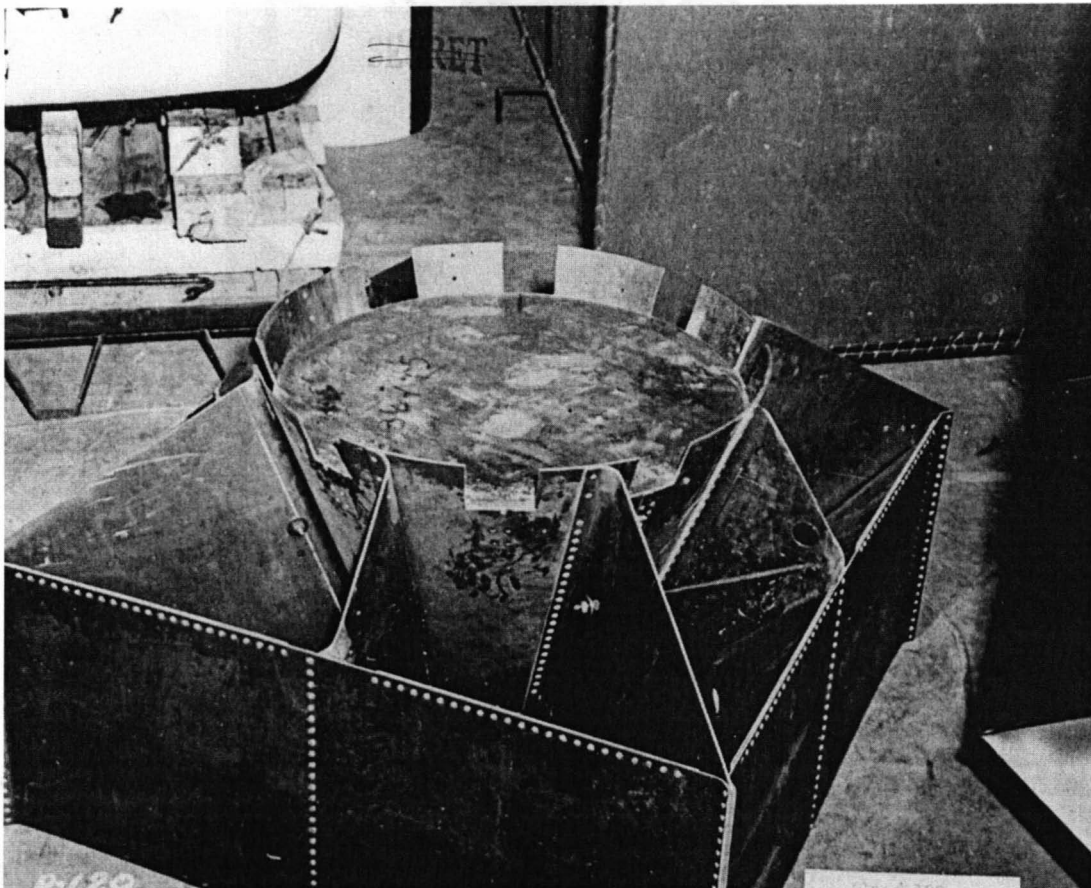
Completed tail fin assembly before attachment to the tail ellipse. (LANL)
