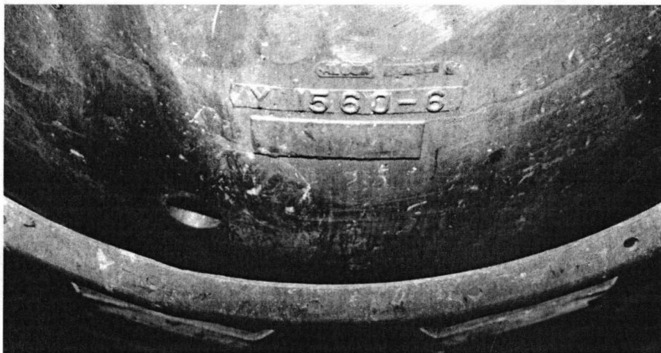
Sphere drawing numbers can be seen cast into the bottom of the polar cap. (Author)
