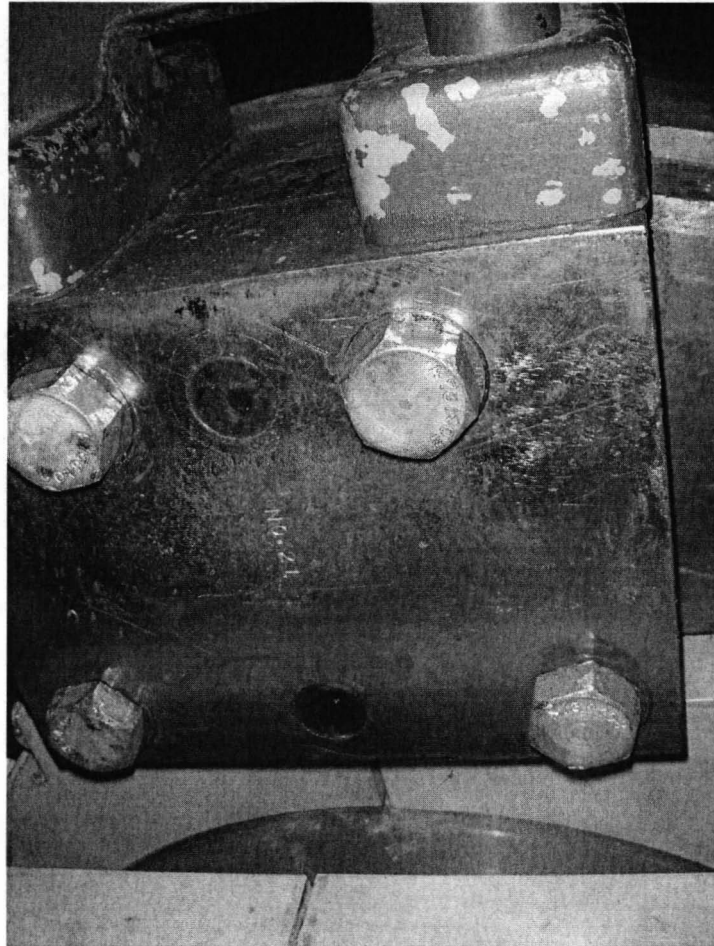
Close-up of the 2" x 5.25" x 6.6875" target case block used to attach the lift lug. Below it are the two splitting locking collars used to attach the battery boxes to the target-case to gun-tube adapter which is visible between the collars. (Author)
