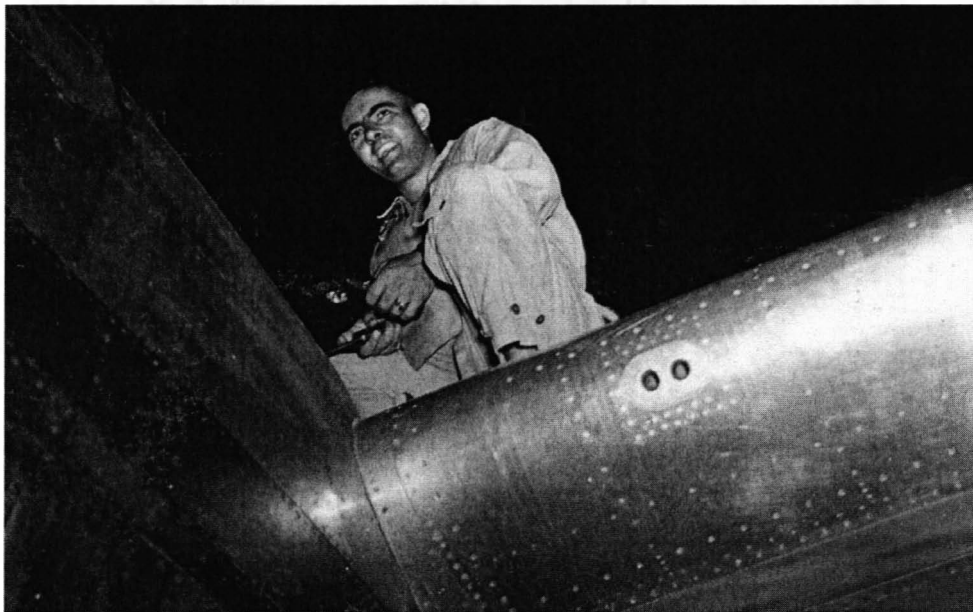
Assistant Flight Engineer Sgt. Raymond G. Gallagher checking fuel tank levels in Bockscar before takeoff. (USAF)
