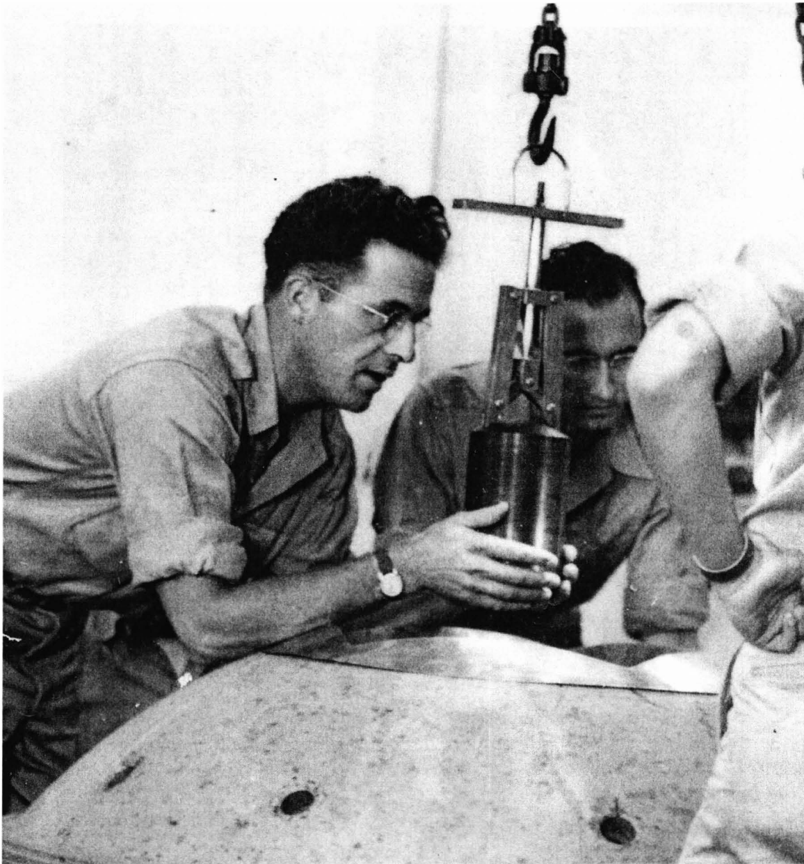
This very rare photo shows Raemer Schreiber steadying the 5" diameter Pu-filled uranium "capsule" as it is about to be loaded into the F-31 Fat Man Dural sphere inside Tinian Assembly Bldg. #3 in 1945. The top plate on this F-31 sphere is the same style as the one used on the Trinity sphere shown on the previous page. This top had a metal funnel built into it to protect the surrounding explosive blocks while it was being loaded into the 8.75" diameter Uranium tamper sphere down in the very center of that sphere. Schreiber was present a few weeks earlier in the McDonald Ranch House to observe the assembly of that same style capsule for the Trinity device. In an extensive 1996 interview, he gave the author a complete description of exactly how that capsule was assembled. (Author)
