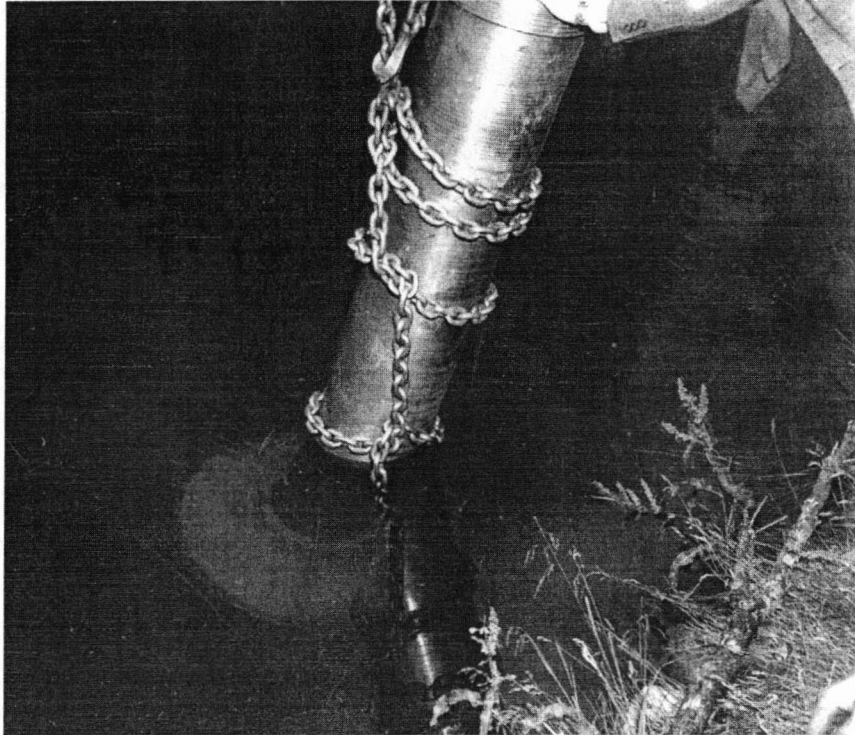
Little Boy gun tube attached to a target case shown submerged in a pond at Los Alamos to test for water leakage through the vent seals at the back of the target-case to gun-tube adapter. Note the scientist (with tie) at the top peering down the gun tube to check for the presence of water in the target case. Two of the four seals are barely visible underwater at the 6 and 9 O'clock positions on the aft end of the target case and the exposed surfaces of the uranium were plated with 0.005" of cadmium for safing the gun in case of immersion in water. (LANL)
