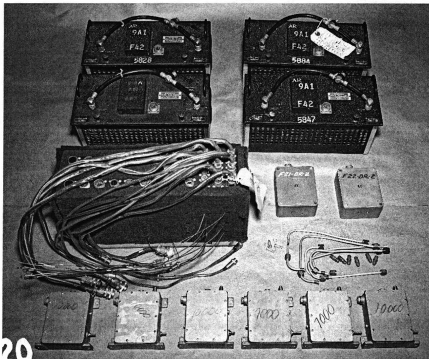
Good view of the X-unit bolted to the "B" plate on the front cone with coax cables going to the detonators. When the front armored ellipsoid ballistic case was attached, the wires shown on the front of the X-unit were attached to the step-up transformers and the inverter. Ballistic case attachment cubes are visible on sphere. Below is a complete set of Firing and Fuzing components for the FM including a Clock Box with cabling, APS-13 radars (4), 0.38 second delay relay (2), and baro boxes (6) with tubing. (LANL)
