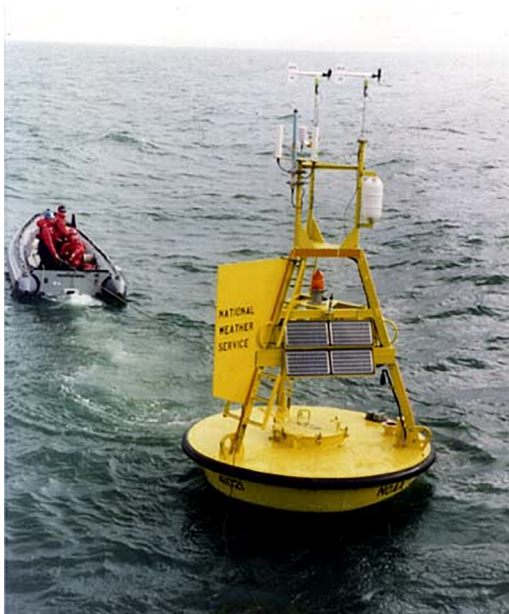
Figure 7.2 A weather and wave buoy operated by the NDBC. Instruments that measure wind, temperature, humidity, and pressure are located on the mast from top to bottom. Accelerometers inside the hull record the wave-induced motion of the buoy, which is used to derive wave height and other properties. Photograph courtesy of NDBC ( http://www.ndbc.noaa.gov ).
