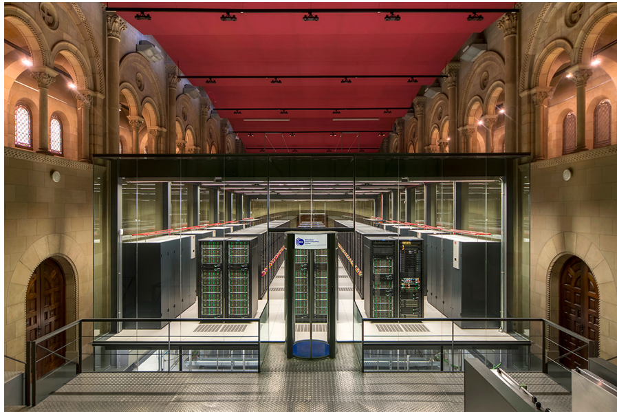
Figure 1.2 The MareNostrum 4 supercomputer at the Barcelona Supercomputing Center. The computer is housed inside the Torre Girona Chapel in Barcelona, Catalonia, Spain. A high-speed network connects all of the cabinets to each other. With 153,216 Intel Xeon cores, MareNostrum 4 is the fastest supercomputer in Spain, and the 37th fastest in the world as of June 2020. ( https://www.top500.org/lists/2020/06 ). It's used for many scientific applications, from astrophysics and materials physics, to climate and atmospheric dust transport prediction, to biomedicine. (Image source: https://www.bsc.es/marenostrum/marenostrum )
