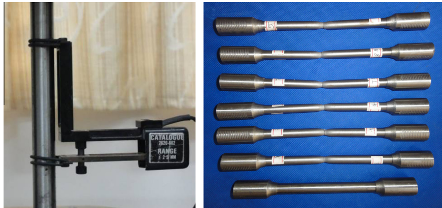
Fig. 3. Standard tensile tests of material specimens.
